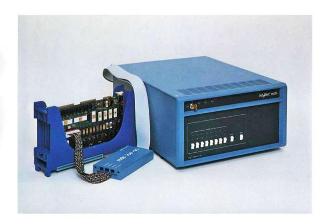
With the powerful Intellec MDS Microcomputer Development System and its ICE-80 In-Circuit Emulator, you can develop and debug your system software directly on the SBC 80/10 ... plus, you can isolate and correct system "bugs" on the production line and in the field
