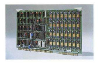
A 16k byte Read/Write Memory Board can be used to expand the RAM memory capacity of your SBC 80/10.
